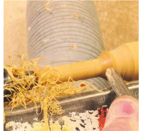
▲ Pic.30 If you turn half a cove after the spigot it will hide the hole where the handle goes into the hammerhead. Before turning the rest of the handle check the fit
